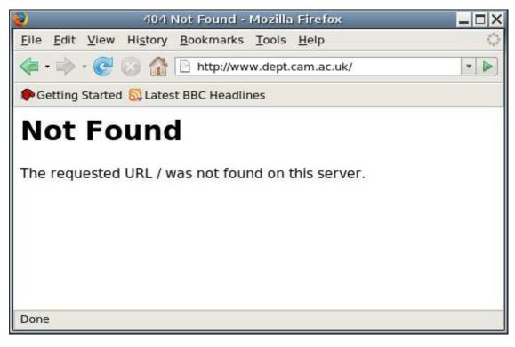
There are two solutions to this issue. The first, and simplest, is to nominate a filename (such as index.html) and instruct that if a directory is requested which contains a file with this name then that file should be treated as the target of the request. This is the approach we will follow in the Section called *Using default documents*.
